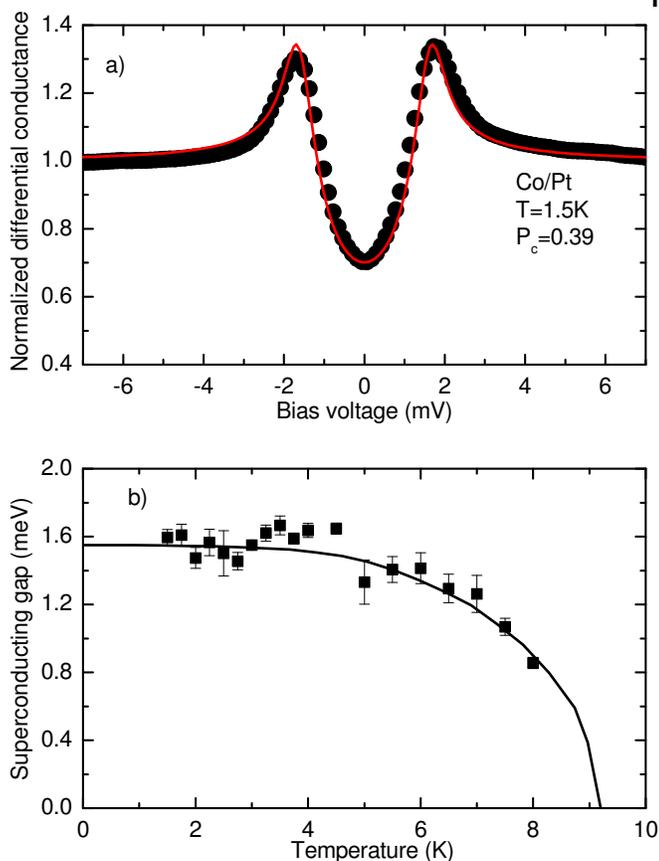
**Fig. 7** Panel (a) demonstrates the differential conductance curve for a nanojunction between a Nb tip and a Co sample with a Pt capping layer. The best fit (red line) yields  $R_N = 780\Omega$ ,  $P_c = 0.39$ ,  $T = 0.87$ ,  $\Delta = 1.62\text{meV}$  at a temperature of 1.5 K. Panel (b) demonstrates the temperature dependence of the fitted gap values clearly following the BCS prediction.
