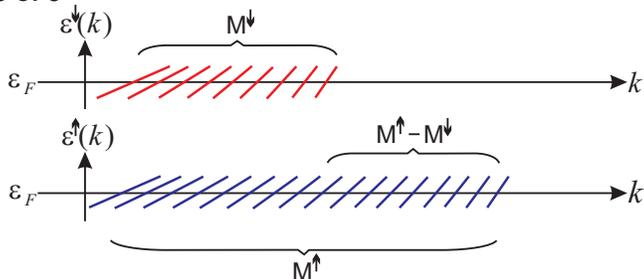
**Fig. 2** The dispersion curves around the Fermi energy for the different conductance channels. The bottom and top panels correspond to spin up and spin down electrons, respectively. Due to the exchange splitting the number of open conductance channels differs for the two spin subbands.
