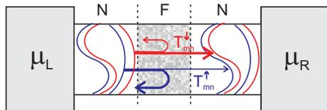
**Fig. 3** A diffusive ferromagnetic region is sandwiched between two normal metal ideal quantum wires. The transport is determined by spin dependent transmission probabilities between the conductance channels at the two sides.
