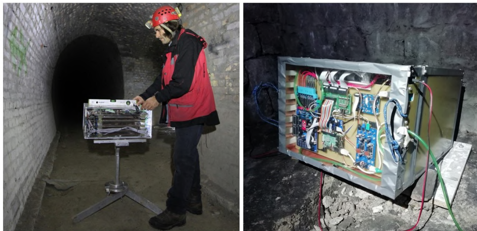
Figure 4.11: Images of the tracking detectors consisting Close Cathode Chambers, installed in the Királylaki tunnel [156].
