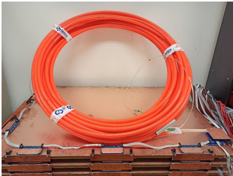
Figure 3.23: The 50 m long 16 mm inner diameter PE-RT buffer tube attached to the end of the gas chain containing eight type 120 MWPC chambers [99].
