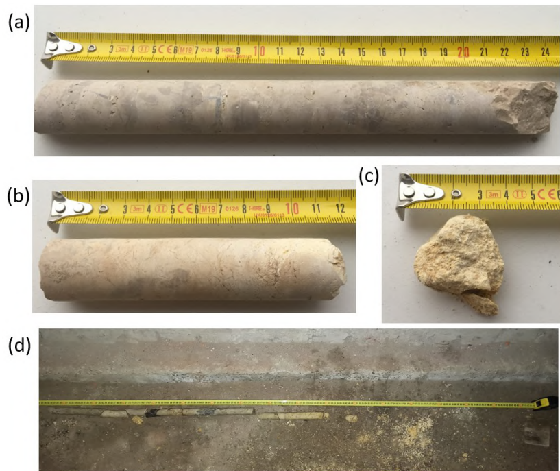
Figure 4.17: Drill cores with different densities: (a) intact cherty dolomite ( 2.6\text{-}2.7 \text{ g/cm}^3 ); (b) slightly altered dolomite close to the walls of the fissures ( 2.4\text{-}2.5 \text{ g/cm}^3 ); (c) altered dolomite powder (less than 1.8 \text{ g/cm}^3 ); (d) the full extent of the last 2 m drill core from one of the drill holes. Dolomite powder only partially recovered [156].
