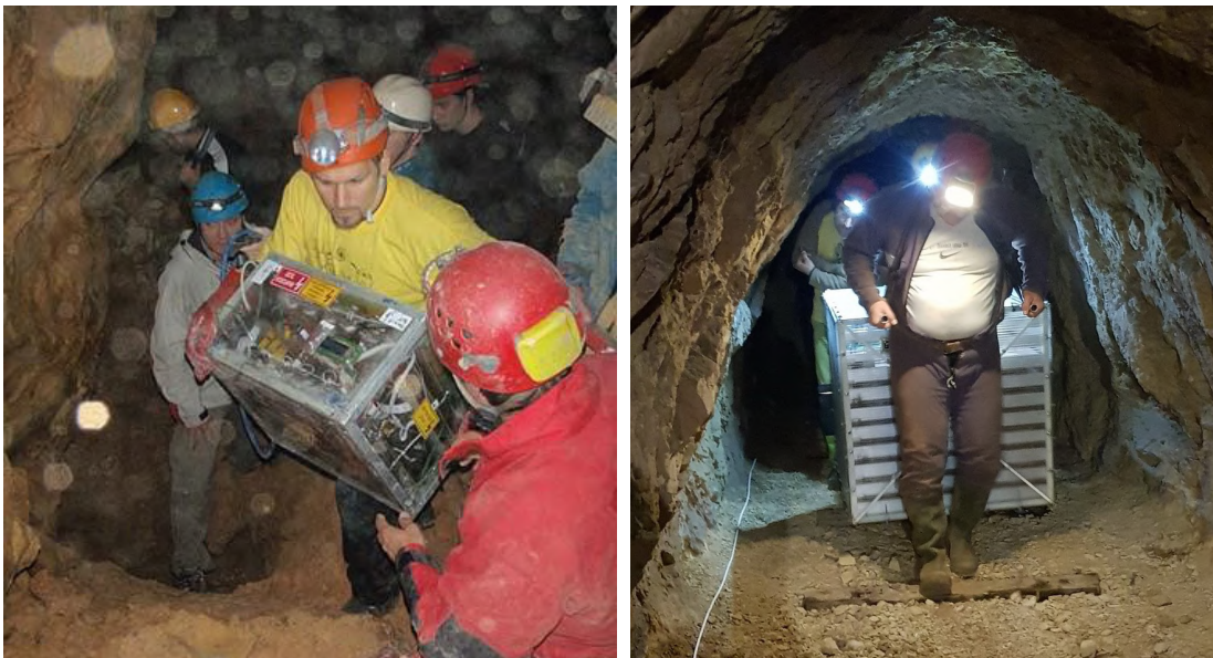
Figure 2.13: Examples of muon detectors installed underground. Left: Photo taken in the Ajándék cave near Budapest, which is a good example for humid environment. Right: Installation in the Esztramos abandoned mine system in Hungary, which illustrates well the limited space and the importance of portability [30].
