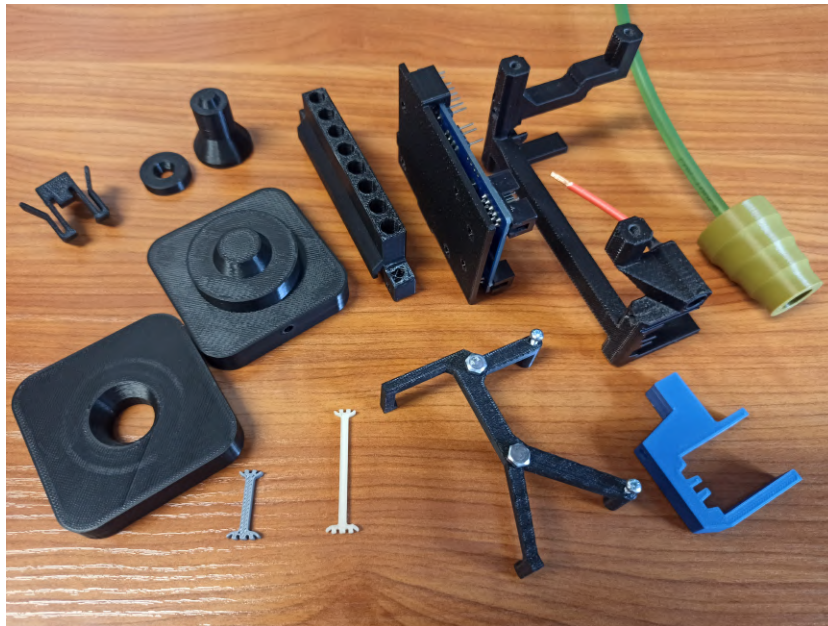
Figure 3.11: Some of the 3D prints designed for special mechanical purposes. The insulating material allows custom designed connectors, and the high precision enables fine-tuning alignment or support components.
