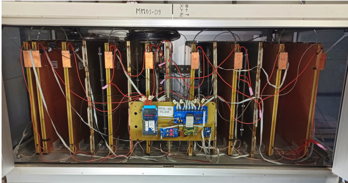
Figure 3.12: A MMOS module at the Sakurajima Muography Observatory [92]. The MWPC modules and absorber/scattering lead walls are arranged vertically, and the DAQ system is located at the center.
